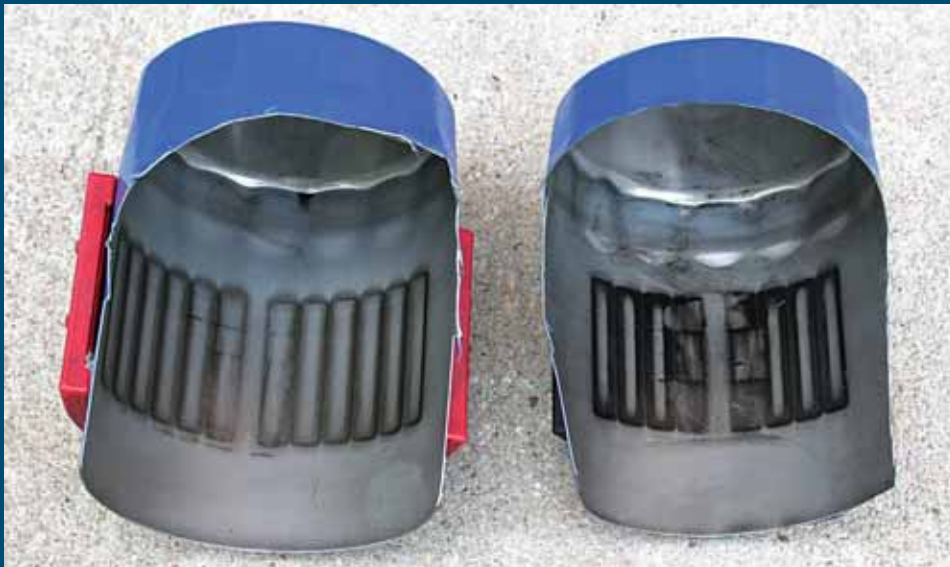
△ The filter on the left came from a Duramax diesel with 40,000 miles, the one on the right from a small-block Chevy with 30,000 miles. You can readily see how the individual magnet elements have trapped and held the small metal particles. While small, you can easily feel the grit when rubbed between your fingers.
